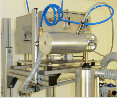
NDF100-BD on top of filter tester (left) NEW dispersing head (top) NEW control unit (right)
