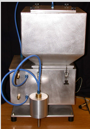
NDF100-3FI on platform balance (top) with additional container (left) with new digital pressure controllers (right)
