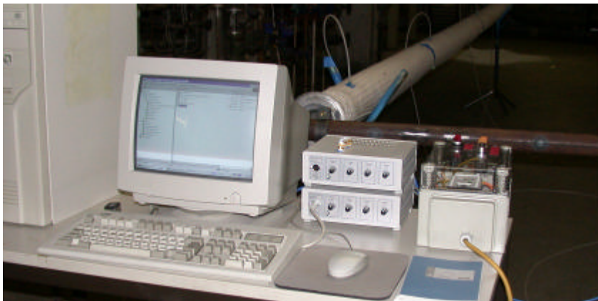
Set-up for one blow tube with 12 filter bags
